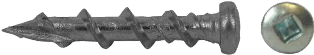
**Multi Screws** are a one piece Class 3 self drilling anchor. Designed to hold strong in masonry, concrete, brick, stone, thick plasterboard and plywood. T17 point to assist with embedment into material. Aggressive “teeth” for an extra strong grip. Unlike most masonry fixings, the Multi Screw can be reversed out and used multiple times.
